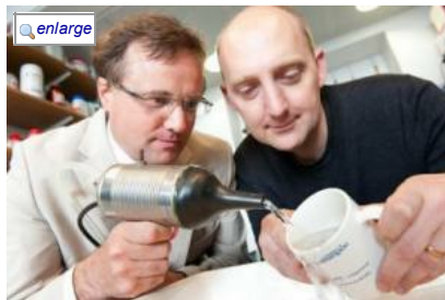
Prof. Leighton (left) and Dr. Birkin with their ultrasonic nozzle device. The revolutionary ultrasonic attachment for taps massively enhances the ability of water to clean. (Credit: University of Southampton)
