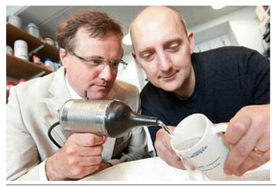
Scientists at <u>Southampton</u> University have developed an ultrasonic attachment for taps and hoses that can enhance water's ability to clean.
