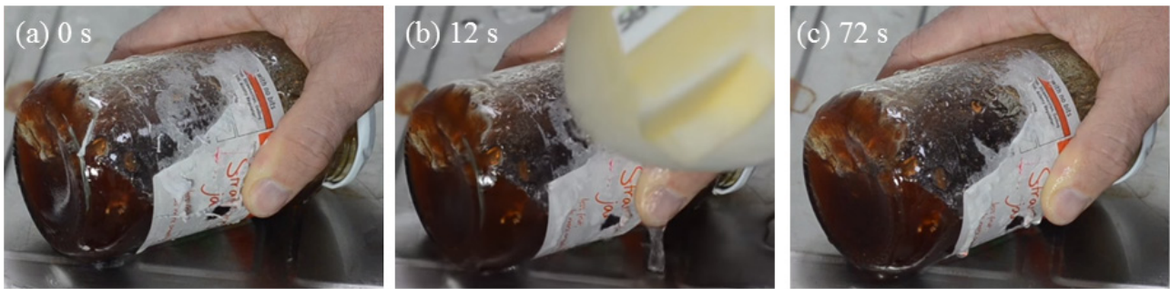
Figure 7. Removal by the UAS of glue used to attach label to jam jar. The video of this is available at https://www.youtube.com/watch?v=0H3ZE9IrgoQ .
